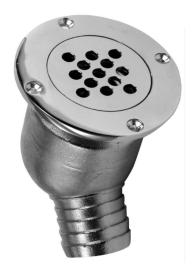
**Description:** 45° cockpit drain with check valve, fitted with check system: an inner ball prevents any backflow. Removable grid for cleaning.
